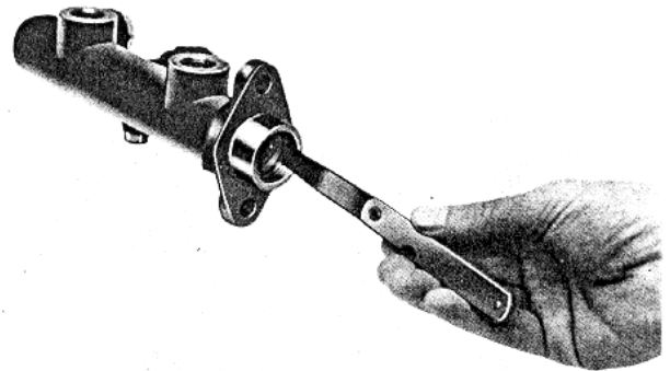
Fig. 11-12 Checking piston clearance
