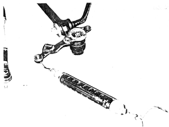
Fig. 13-33 Checking revolving torque
