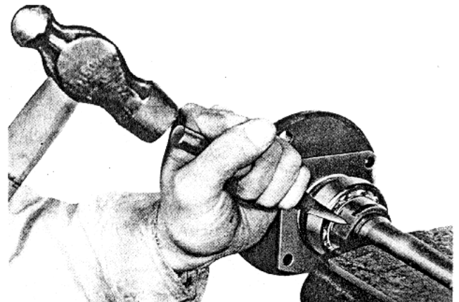
Fig. 9-4 Cutting bearing retaining collar
