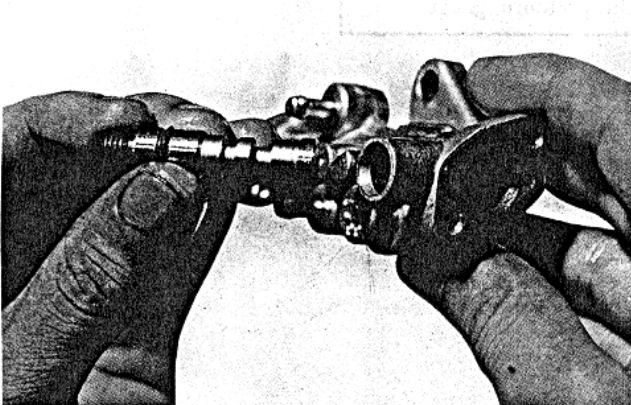
Fig. 2-27 Inserting control pin
