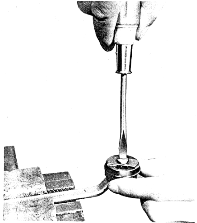
Fig. 13-9 Disassembling base valve assembly
