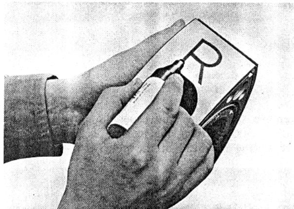
Fig. 1-23 Putting identification mark
